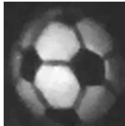
Right: image taken by a one-pixel camera using 1,600 shots.
